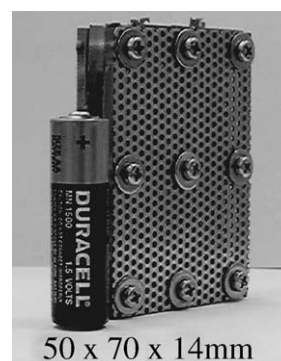
Fig. 11. Small air-breathing DMFC cell pack with four unit cells.
